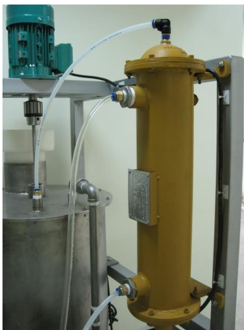
Figure 3. Methanol recovery system.
